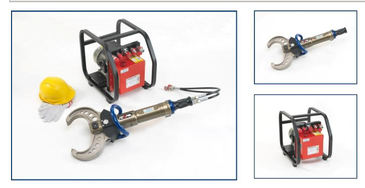
The set is formed by a concrete cracker and a hydraulic power pack that can have three different type of motors : electric, gasoline or hydraulic. The use of the set is ideal in all controlled demolition works and in the emergency rescue operations after concrete structures downfalls. The cracker with incredible power, without vibrations and dust formations walls in reinforced concrete or bricks, floors, pillars, stairways and other concrete or composite structures.
